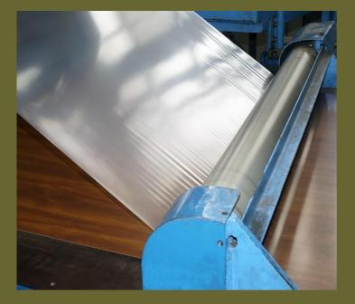
The SMP Coil Coating has excellent Long Gloss retention. It is Proprietary High Durability Polyester Resin modified with Silicon for resistance to chalking and facing. It is Corrosion protecting in severe environments.
